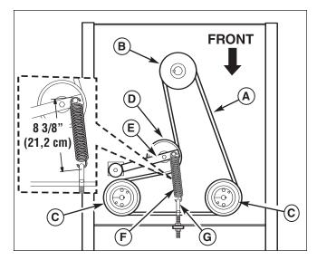
Figure 43. Hydraulic Pump Drive Belt Replacement
